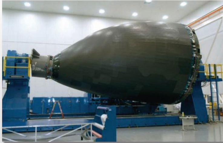
Boeing 787 composite nose being manufactured (width: 18 ft 11 in (5.77 m))
